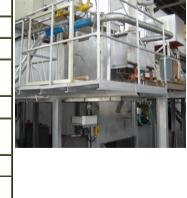
TE CBF 1000-1500 lines are the core of CBF production plants with output capacities of 3 000/5 000/10 000/15 000 tons a year.
